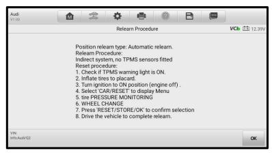
Figure 6-12 Relearn Procedure for Indirect TPMS
