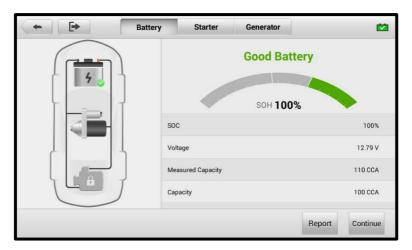
Figure 13-7 Battery Test Results Screen
