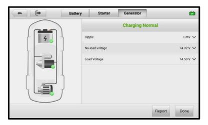
Figure 13-9 Generator Test Results Screen
