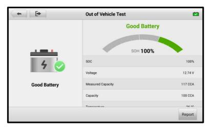
Figure 13-11 Out-vehicle Test Results Screen
