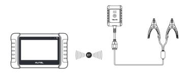
Figure 13-3 Battery Tester Connection Example 1
