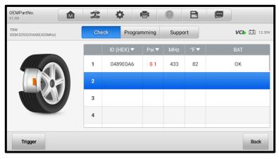
Figure 6-43 Check Screen via OEM Part NO.
