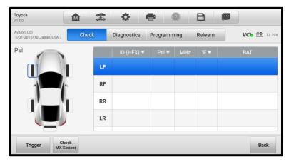
Figure 6-13 Relearn Procedure for Direct TPMS
