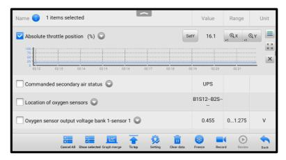
Figure 4-15 Waveform Graph Mode Screen
