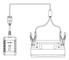
Figure 13-4 Battery Tester Connection Example 2
