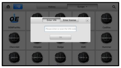
Figure 6-5 Manual Input in TPMS Application
