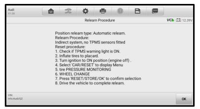
Figure 6-12 Relearn Procedure for Indirect TPMS
