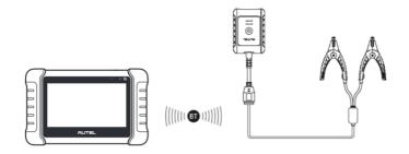
Figure 13-3 Battery Tester Connection Example 1
